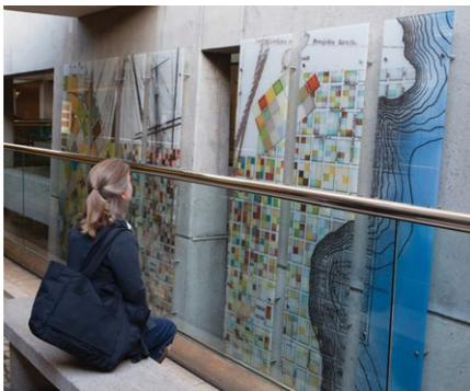
or artificial lighting. The inks offer enhanced resilience against chemicals and UV, on top of the extreme durability that all Dip-Tech inks possess, so architects and fabricators need not be concerned with printing on the exposed side of the glass.
